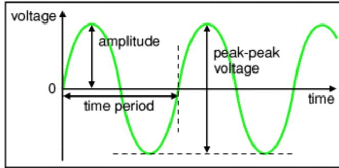
Figure 3: Characteristics of a voltage wave form
