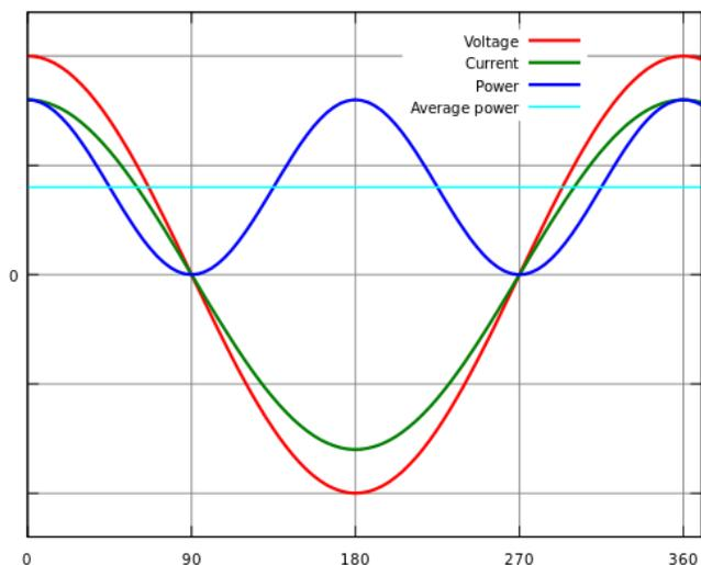
Figure 4: In-Phase Voltage and Current Wave Forms
