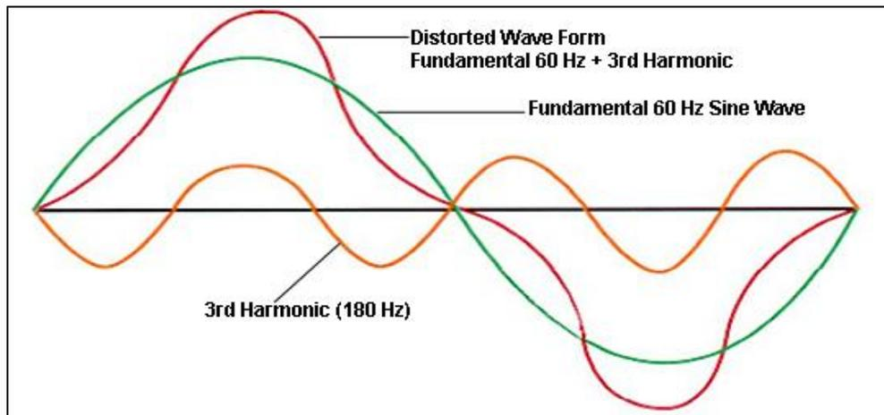
Figure 6: Distorted Waveform Composed of Fundamental and 3<sup>rd</sup> Harmonic. THD approximately 30%
