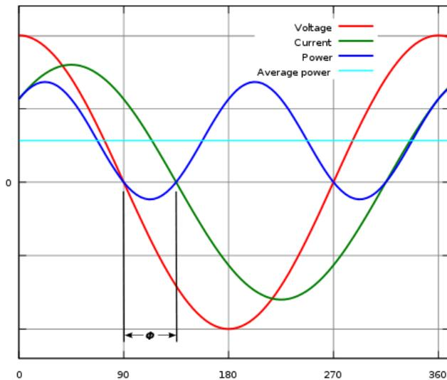
Figure 5: Out-of-Phase Voltage and Current Wave Forms
