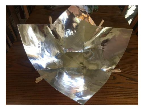
Raise each panel up. Form a funnel by overlapping the panels with one another. Join together with a sturdy clip.
