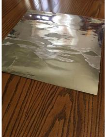
Examples of reflective material: aluminum foil, self adhesive vinyl, and the interior of chip or snack bags. Material can be applied with glue.
