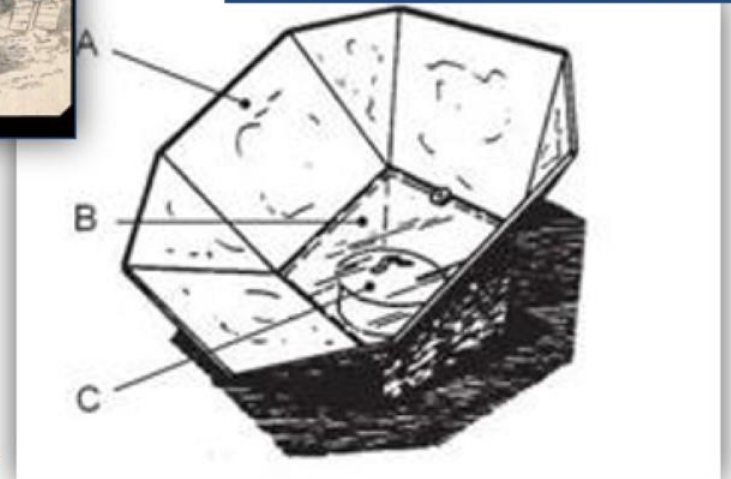
W Adams 1878 Bombay, India Eight mirrors reflect light into wooden box.
