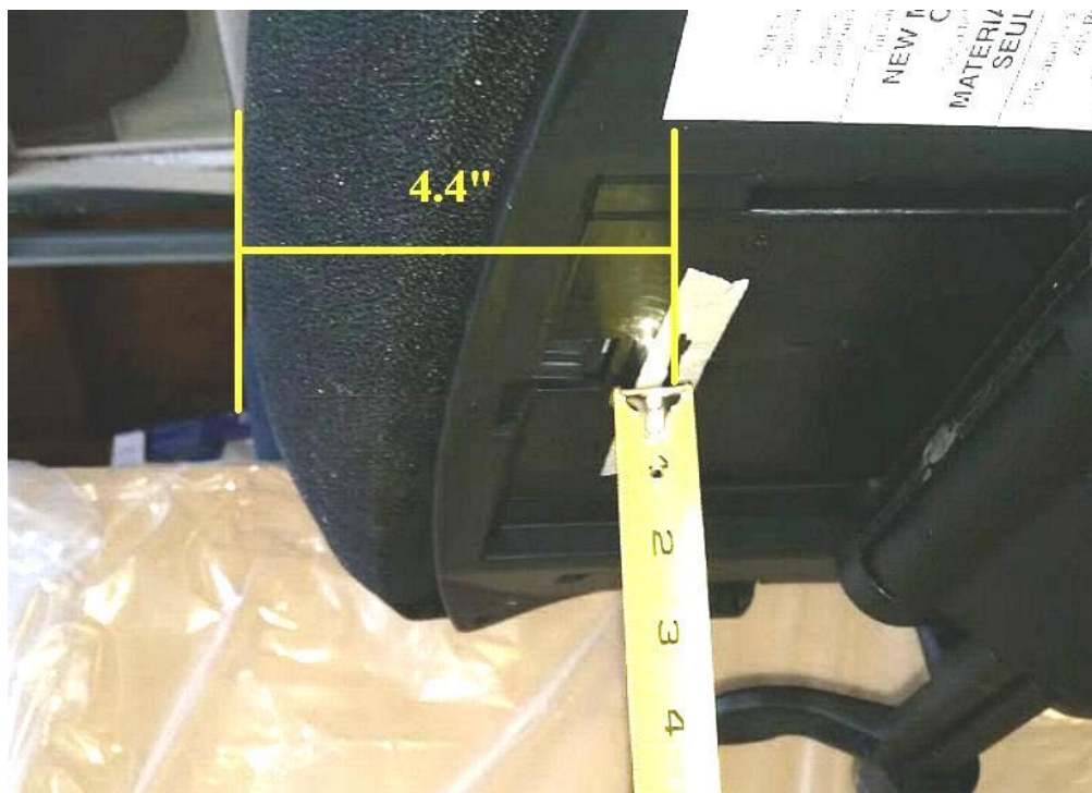
Tape with the line is at 4.4" back from the front edge, the same as the loading point.
