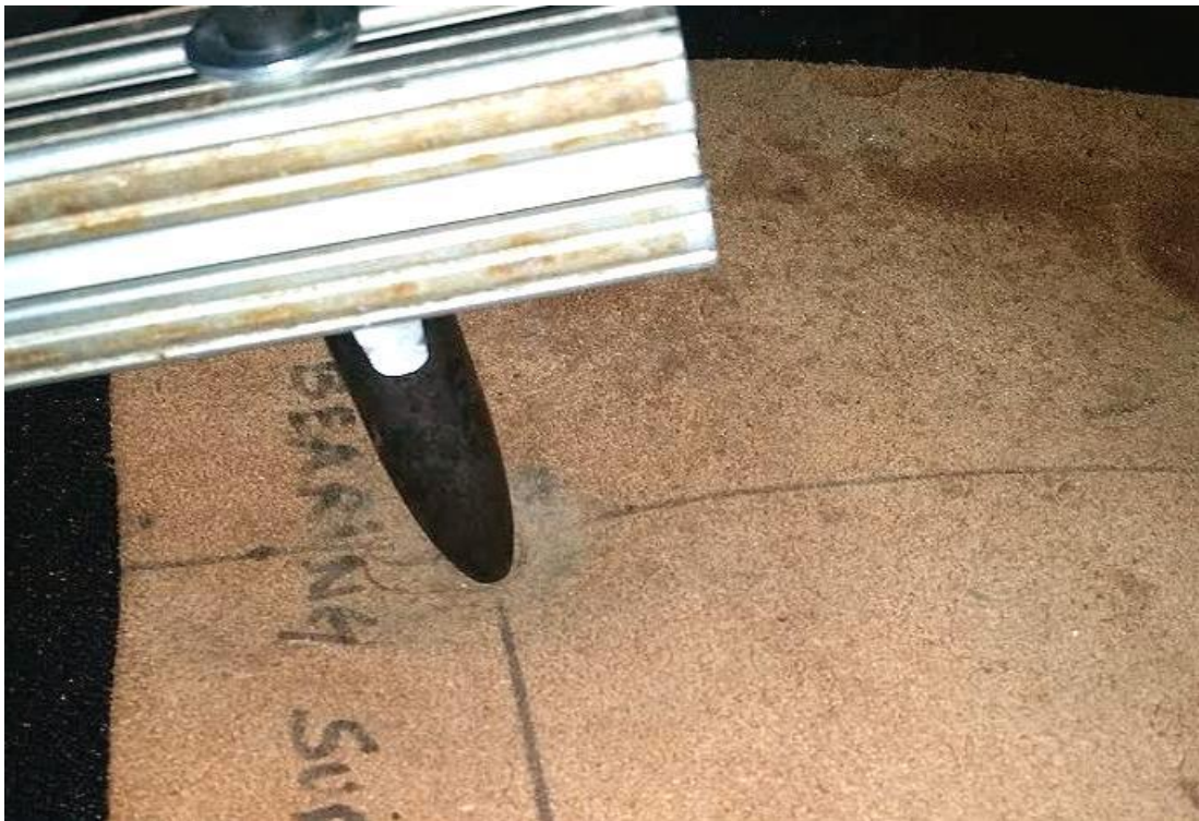
Forward Stability test fixture placed at 2.4" loading point, or 4.4" back on this chair
