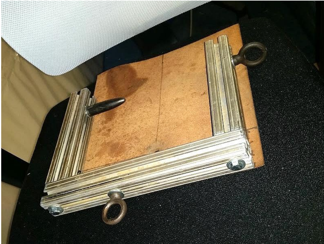
Forward stability test fixture
