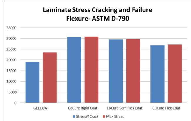
Figure 2: Comparison of laminate stress cracking and failures in flexure for conventional gel coat and Co-Cure coating configurations.
