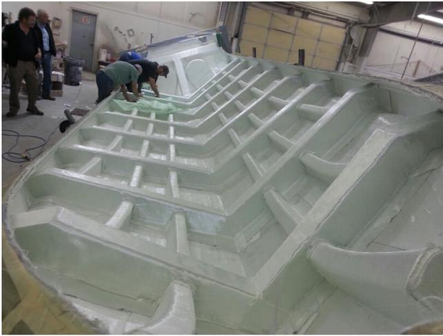
Figure 5: SBIR Phase III 11M low cost lightweight shock mitigating prototype combatant craft hull in fabrication.
