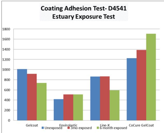
Figure 3: Coating adhesion test results comparison for estuary exposure of coatings.
