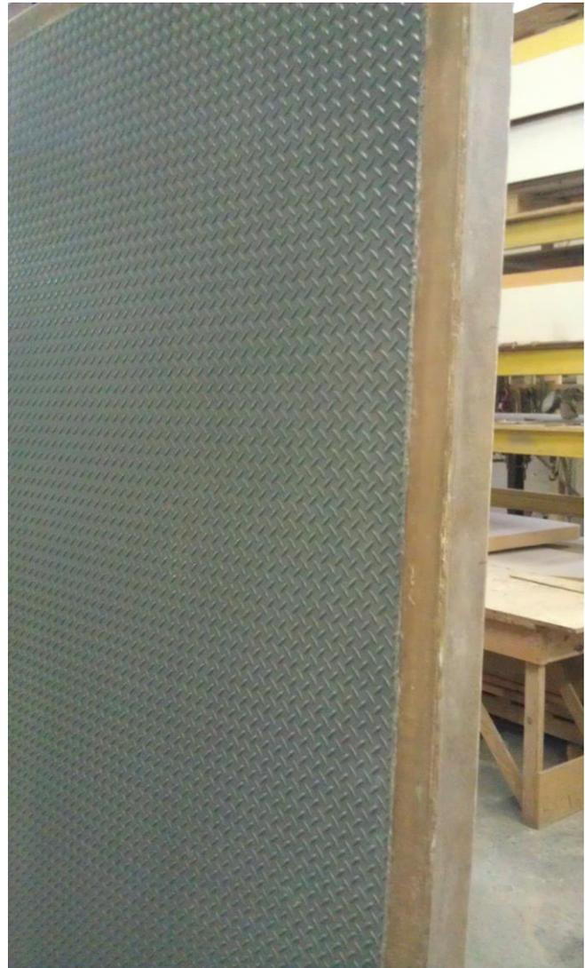
Figure 4: Co-Cure coating as a wear surface for a prototype produce box truck.
