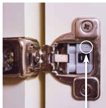
The Soft Close feature is ON when the switch is towards the "-" symbol.
