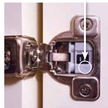
The Soft Close feature is OFF when the switch is towards the "O" symbol.
