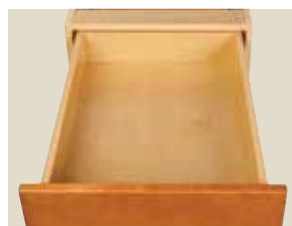
DRAWER BOX 5/8" thick plywood with 3/16" thick plywood captured bottom panel. Full Extension Soft Close runners.**
