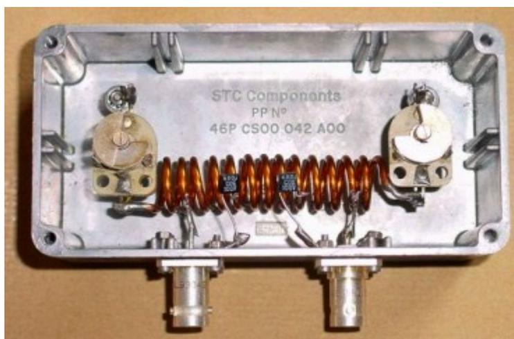
Alignment is a simple process: connect the filter between a transmitter and VSWR meter, and attach a dummy load to the filter output.
