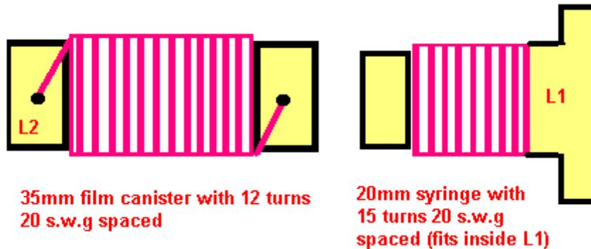
This simple aerial tuning unit is a useful modification of the Z match. It uses a parallel circuit for 30 - 80 and a series tuned arrangement for the bands up to 10 metres. The mode of operation is selected by a DPDT switch.
