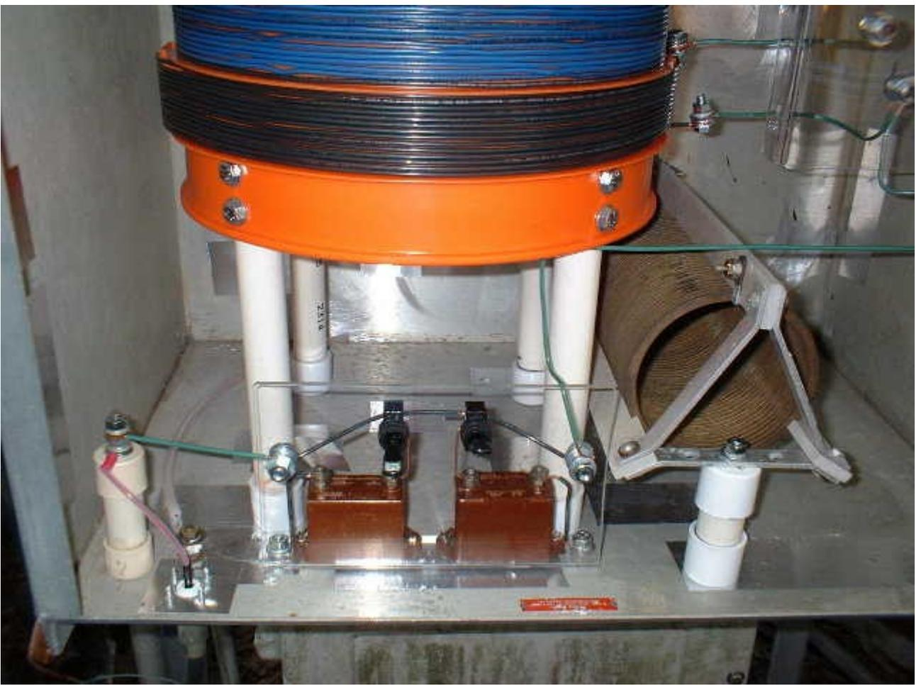
A closer view of the capacitor switching assembly. The capacitors are surplus Mica capacitors rated at 5000 volts. They were made in about 1946, and still work perfectly. The switches came from Radio Shack, and are rated at 12 volts DC, but I tested them at 300 volts RF and they worked fine. No, I did not hot switch them, but the insulation handles the open circuit voltage OK.
