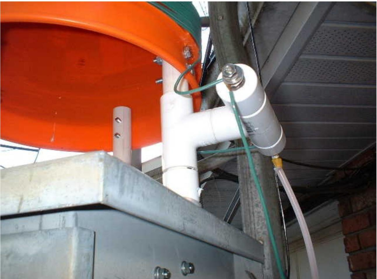
A close up view of the "T" insulator. It's made from a couple of 3/4" PVC pipe tees and a few 2" long sections of PVC pipe, all glued together. Be sure to put the bolts through the pipe caps on the end of the insulator BEFORE you glue the
