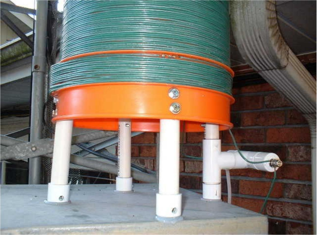
Another view of the LF loading coil mounted on top of the tuning cabinet. Look at the cheap but effective "T" insulator on the right hand leg. This insulator holds both the leads from the loading coil firmly in place.
