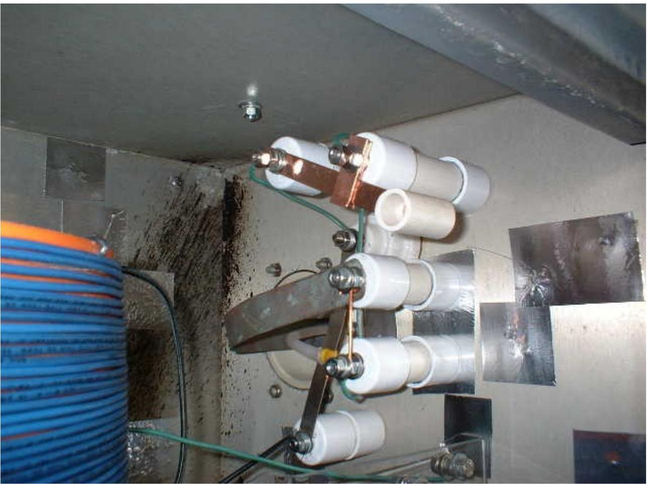
A view inside the cabinet from a different angle. Here you see the LF loading coil bypass switch in the closed position for MF work. The switch is made from sections of flattened 3/8" diameter soft copper tubing. I hammered it flat and pounded it to work harden it.
