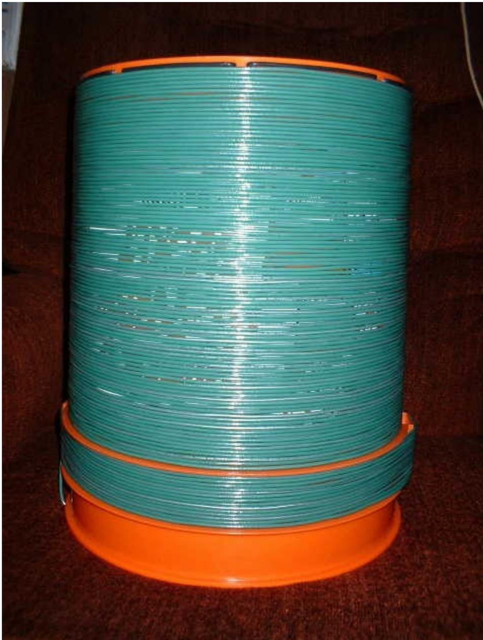
I decided to build a new loading coil instead of using the existing tapped coil which resulted when I split the original double-bucket variometer into two parts. I wanted to keep the tapped coil unit for other tests, and I did not need any taps on the "final version", shown here. Note that I added another 14 turns of wire on the lower end of the bucket. I figured that I could use a little more inductance in this coil.
