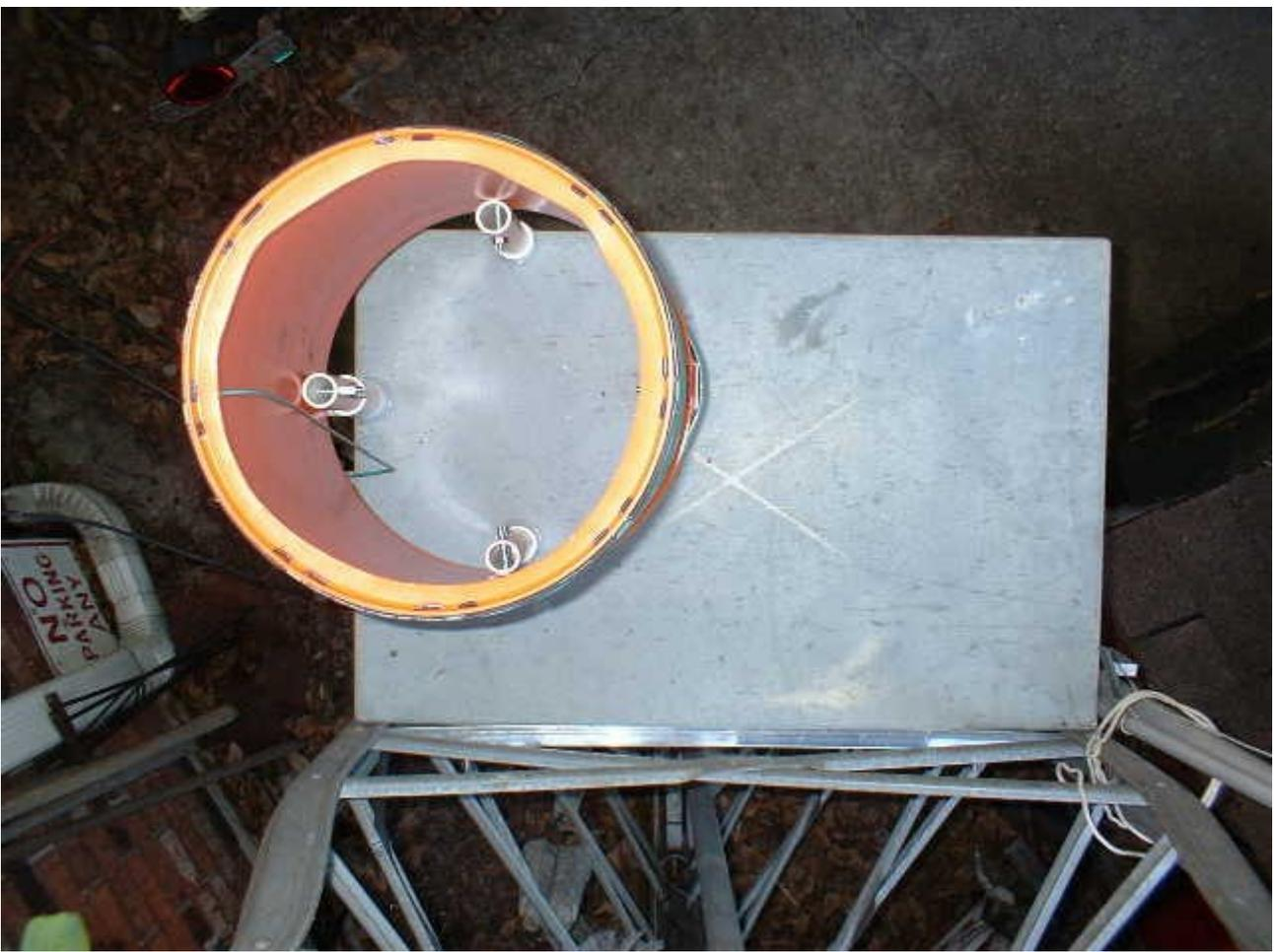
Looking down at the top of the LF loading coil and the antenna tuner cabinet. I have cut the end out of the bucket. Here in south Louisiana, any nice, dry place, such as under an upturned loading coil bucket, tends to collect wasp nests in abundance. Hence, cutting the end out of the bucket may be regarded as an operator safety precaution! Notice that the top coil wire which eventually connects to the antenna, is spaced away from the bucket wall by several inches.
