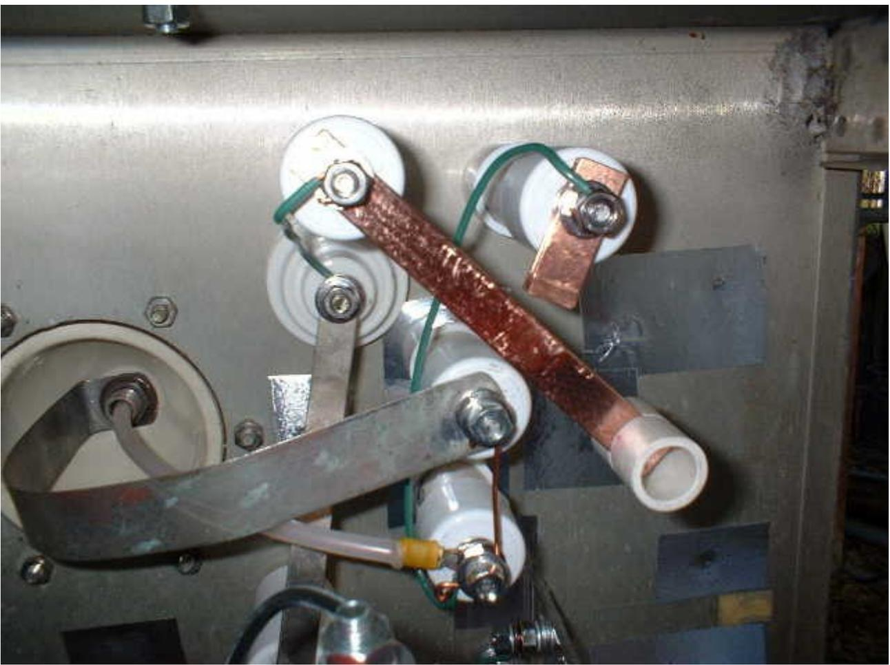
Inside the tuning cabinet, looking at the right side wall. The large bowl insulator is to the left of the picture. I pulled an interesting design trick here. Since I wanted to have the antenna current ammeter located inside the tuning cabinet, that meant that I would have to run the output lead of the LF loading coil back into the cabinet, through the RF ammeter, and the back out of the cabinet.
