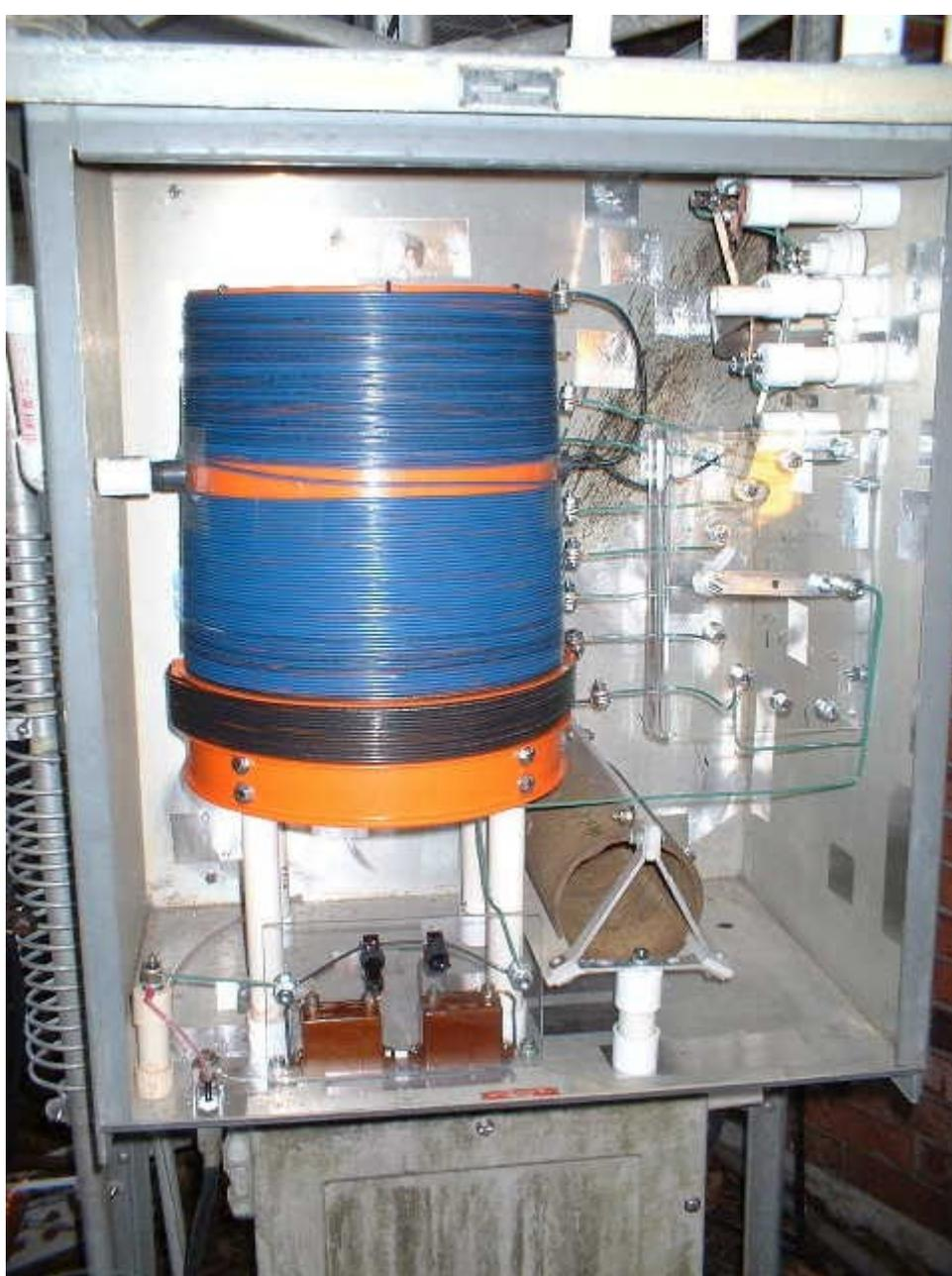
This is what the guts of the completed antenna tuner looks like. The variometer coil itself is inside of the blue and black coil on the orange drum. Note the variometer adjustment handle which passes through the left side wall of the tuning cabinet. The large brown colored coil to the bottom right of the variometer is not used at the present time.
