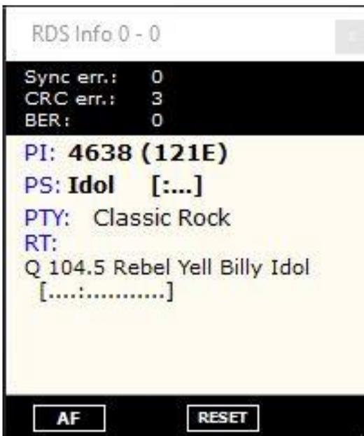
This is the RDS decode window, it will display the PI Code, but currently does not decode the PI and it will give you the text.
