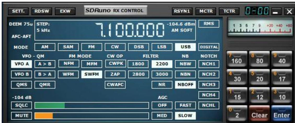
It may look complicated, but it is rather simple, Standard Controls for VFO A/B, Modes, Filters, S-Meter, Band Buttons, AGC, Squelch, Volume, Notch.
