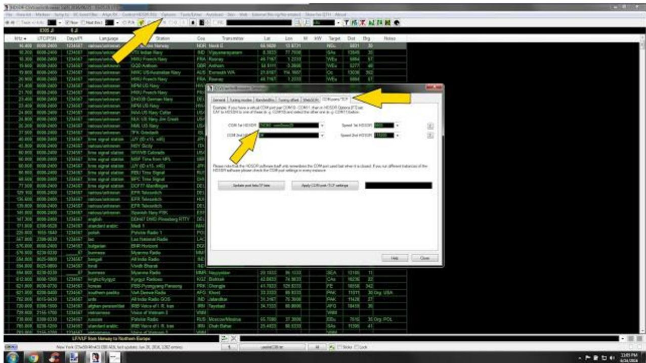
Step 5: Click on "Options" again and select "Settings". Inside of "Settings" select the tab called "COM ports/TCP". This is the sections we will need to know our second assigned com0com port. Inside of "COM ports/TCP" go to the area label COM 1st HSDR and in the dropdown box select the 2nd of the pair of virtual com ports created by com0com. From my virtual pair I chose CNCB0. None of the other settings need to be change. Now click the Close button.
