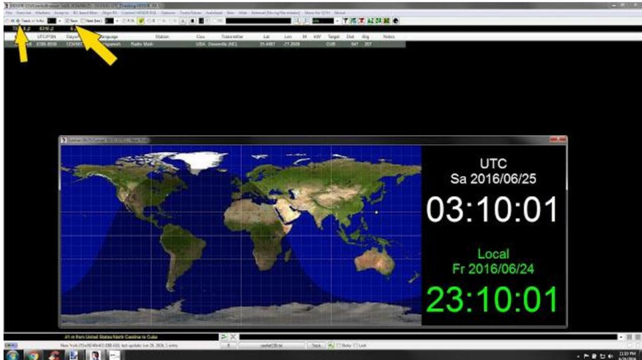
Step 6 Final: On the main screen of CSVUserlistBrowser make sure the Now button is ticked and the next time you load CSVUserlistBrowser along with SDRuno you only have to hit the Track button on the top left. SDRuno will send frequency information to CSVUserlistBrowser and CSVUserlistBrowser will display whatever is on that frequency for that scheduled time.
