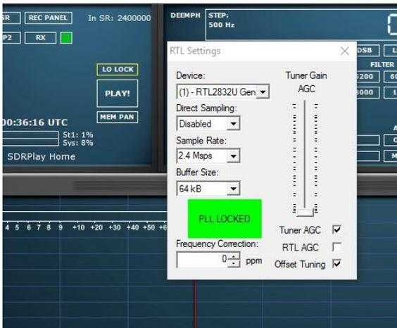
There is a known issue with the RTL extio's at the moment, the drop down menus do not work, but if you click on the sample rate, you can use the up/down keys to change the settings, the AGC slider does work OK
