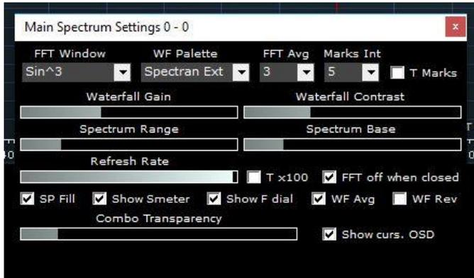
This is the **SETT** window for the SP1, as you can see it has various settings, for the FFT, Palette FFT AVG, Marks is the Time Marks, Range and Base allow you to alter the top and bottom ranges, Refresh rate is the speed of the waterfall
