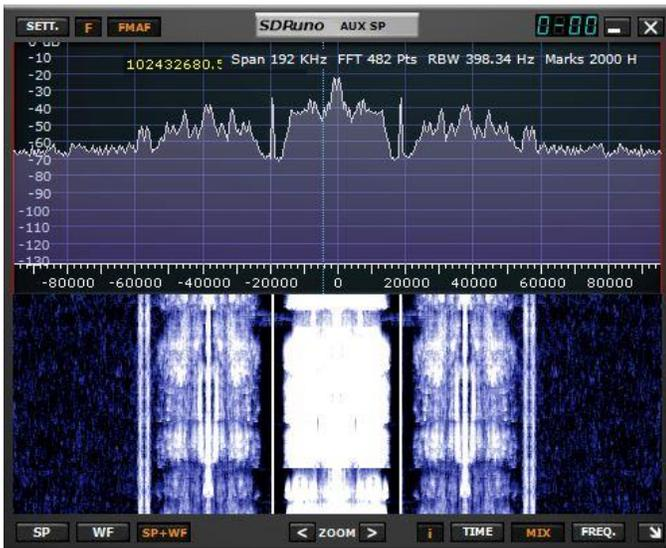
4. Click on the **SP2** Box this is the auxiliary spectrum, where you can look close in at the signal you are on and also vary the filter bandwidth by dragging the filter edges.
