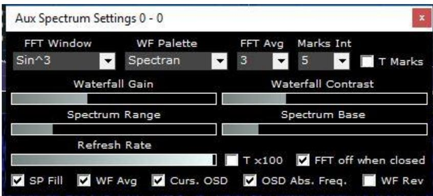
Same controls, FFT, Palette, Contrast, Gain, Range & Base, Refresh Rate, SP Fill, the time marks can also be turned on and off for the SP2 screen, Marks Int is the time interval in seconds, then check the T Marks box for the time lines to appear.
