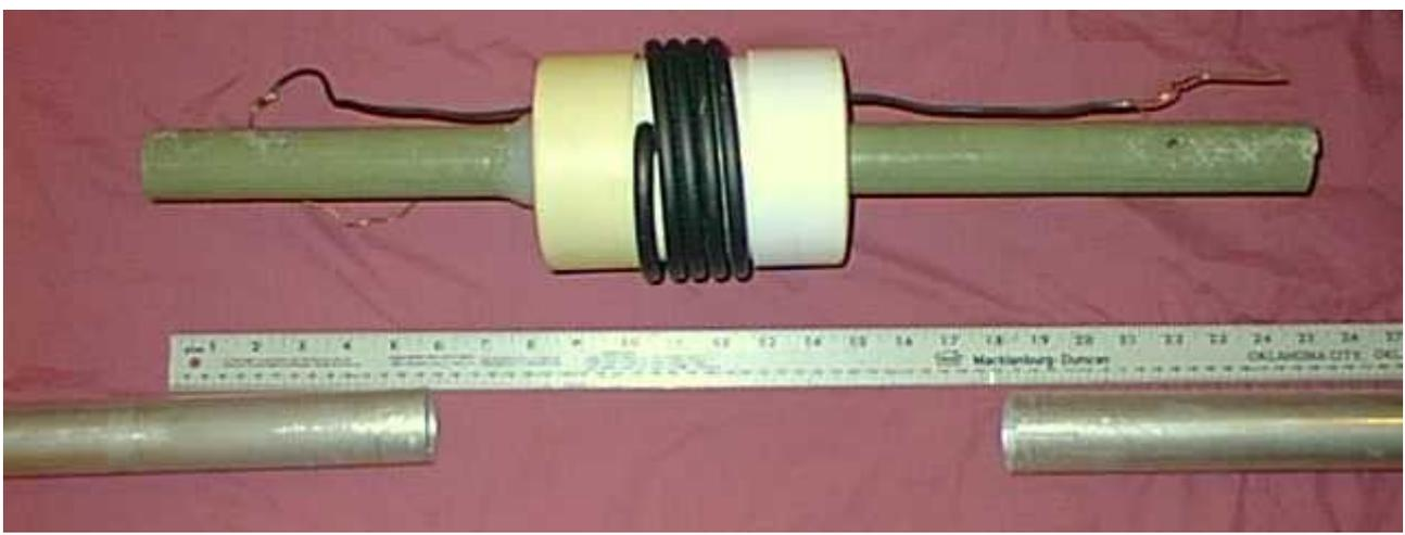
Prototype Coaxial Trap
