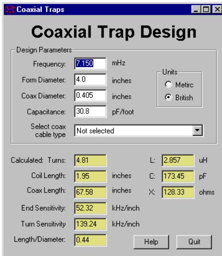
Screen Capture of the Coaxial Trap Design Program
