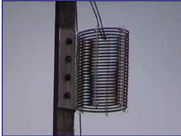
Loading Coil mounted on the 160 Meter Vertical Antenna
