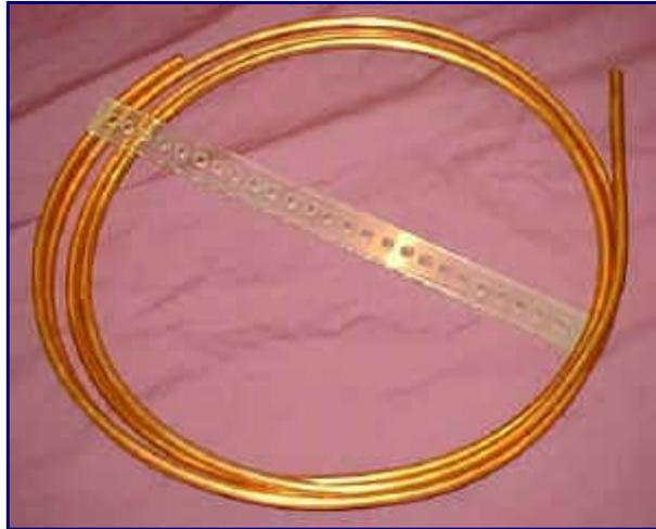
Coil Building Materials, Lexan Spacer Bar and Copper Tubing
