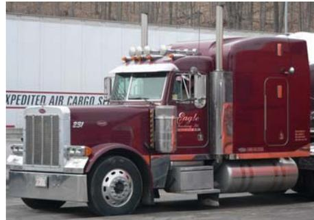
A typical intercity tractor-trailer idles an estimated 1,830 hours per year, during operator rest periods. In North America, there are nearly 480,000 long-distance trucks. For one truck, idling hours can use almost 6,000 litres of diesel fuel per year and give off 21 tonnes of CO<sub>2</sub>, 120 kg of NO<sub>x</sub> and 21 kg of CO emissions.
