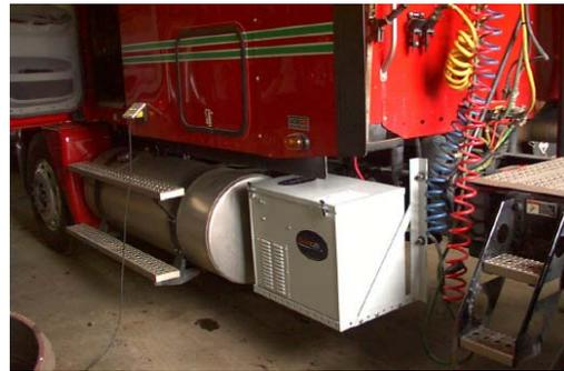
The Novacab system used waste heat to charge the system for heating, so the additional energy required by the system was negligible, except for extreme conditions. Extra electrical energy was required to charge the system for cooling. Using a high-efficiency thermal storage technology (based on phase change of specific materials), with a very high-energy storage density, the climate control system operates independently of the internal combustion engine as follows:
