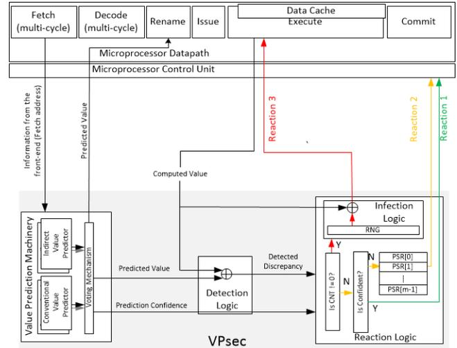
**Figure 1: VPsec high-level diagram. CNT represents the PSR value for the value predicted instruction.**
