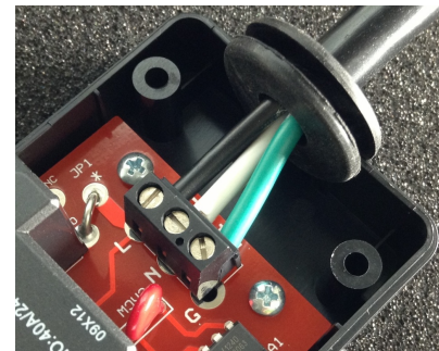
Fig 2: Line cord attached to optional terminal block J2, US/Canada cord.
