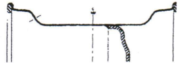
DH style rim with flange reinforcements and formed disc.
