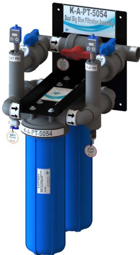
**Mechanics:** Functions by inlet water pressure delivering 35 GPM, and 30-120 PSI pressure. Digital pressure sensors are powered by SWT Municipal Boost Pre-Treatment Monitor System.
