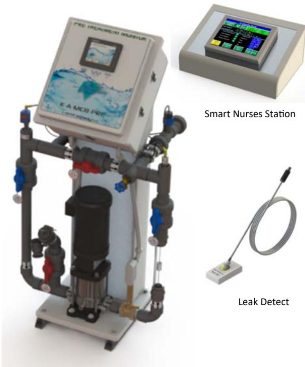
**Mechanics:** Requires Inlet water piping capable of delivering 35gpm for a 2HP pump, 50gpm for a 3HP pump and 30-40 PSI pressure.
