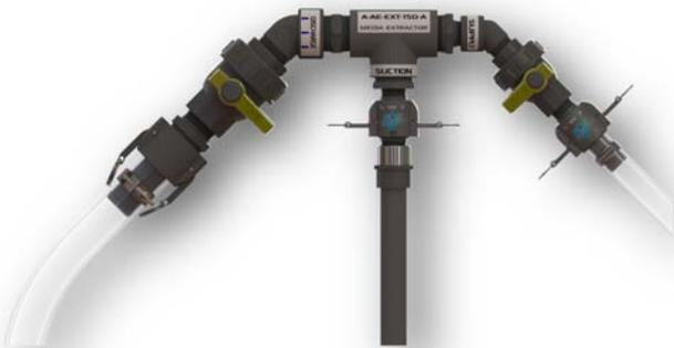
**Mechanics:** No electrical required. By passing water across the extraction tube, a suction effect will take place and pull the media from the tank.
