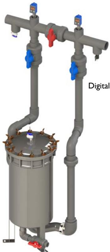
**Mechanics:** Functions by inlet water pressure delivering 35 GPM, and 30-120 PSI pressure. Digital pressure sensors are powered by SWT Municipal Boost Pre-Treatment Monitor System.
