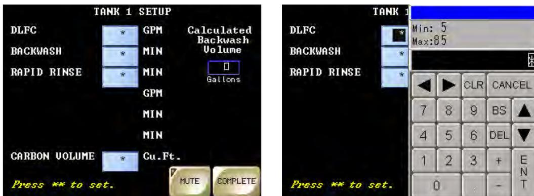
**DLFC- Drain Line Flow Control:** Is a flow restrictor placed on the drain line of a media tank controller to control the backwash volume Fig 3. The DLFC should have a GPM value stamped, stenciled, engraved or inked on side of device. See Fig 4.
