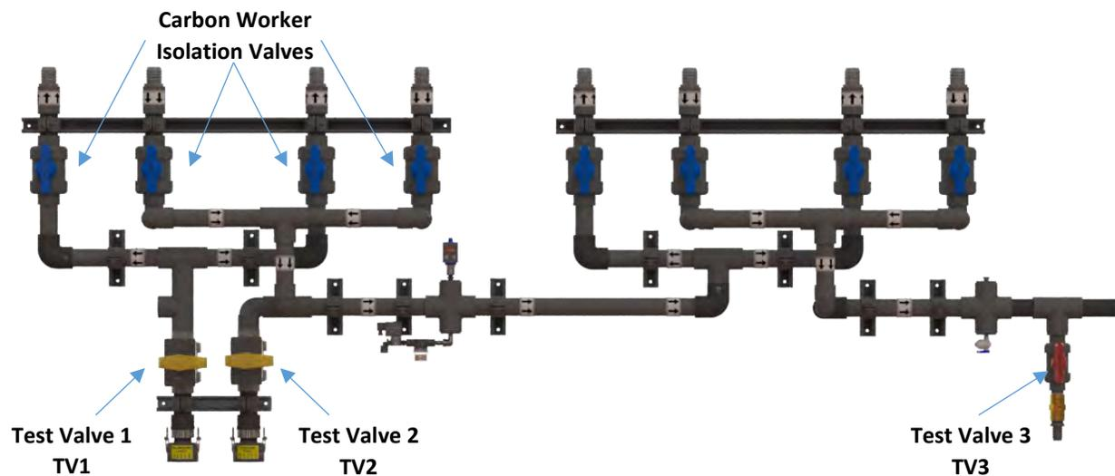
4. Locate the following valves: "Carbon Worker Isolation Valves" - rotate valve handles to the "CLOSED" position.
