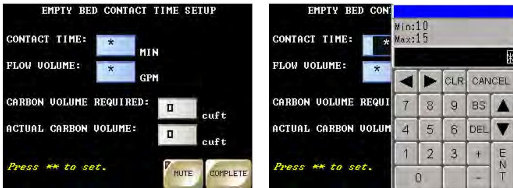
**Contact Time:** Enter your facilities standard for Empty Bed Contact Time. A.A.M.I. Standard is 10 Minutes.
