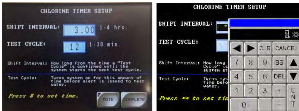
**Shift Interval:** Is the amount of time between the last completed "Chlorine Test" and when the next "Test Cycle" is initiated.
