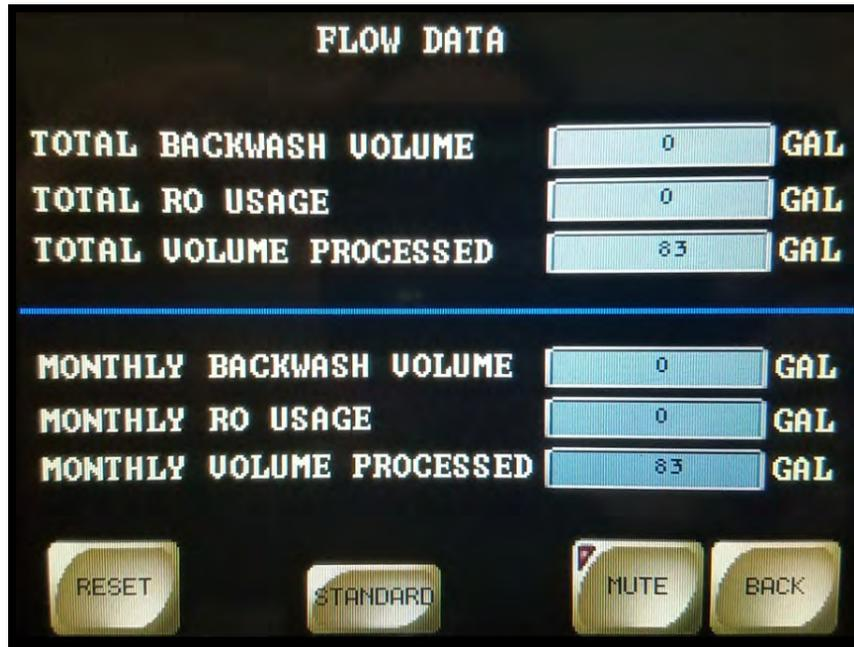
System water usage is monitored at the **FLOW DATA SCREEN**. The values of **VOLUME PROCESSED** are obtained by adding together the water consumed by the cycles (**BACKWASH**, forward flush and regeneration) of the media tanks and the **RO USAGE**.
