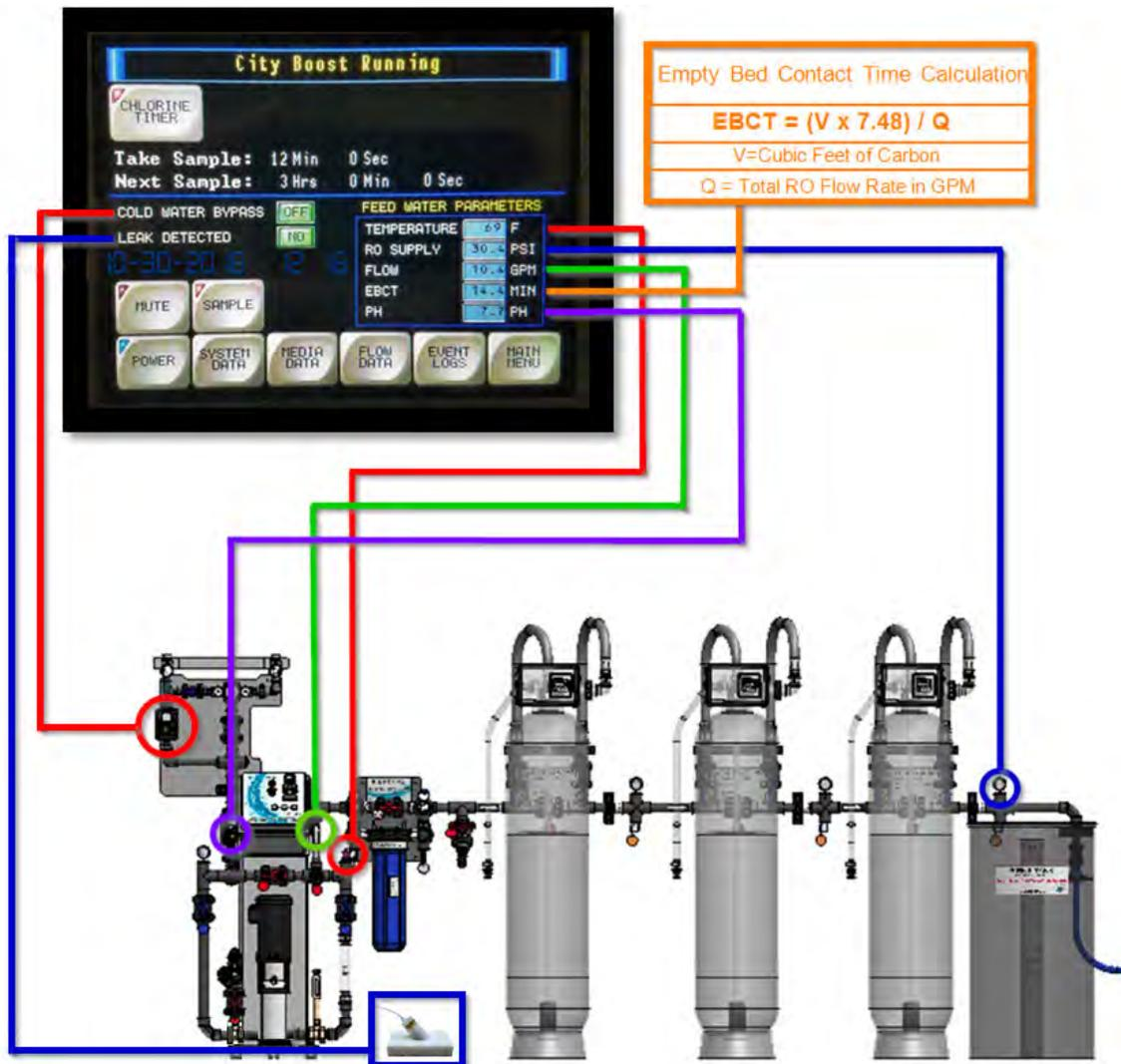
**COLD WATER BYPASS:** Automated valve position is monitored and displayed.
