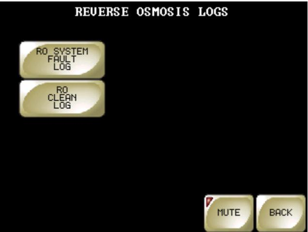
**RO SYSTEM FAULT LOG:** Records the dates and times of the alarm states transmitted by the reverse osmosis machine.
