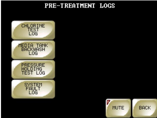
**CHLORINE TEST LOG:** Records the dates and times of completed chlorine test cycles.
