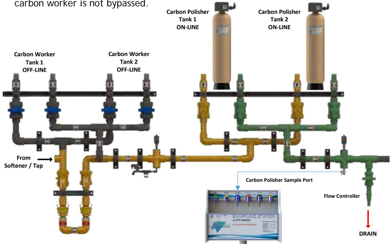
6. Install "Worker Bypass Shunt" as shown. Make sure cam levers are in the locked position.
