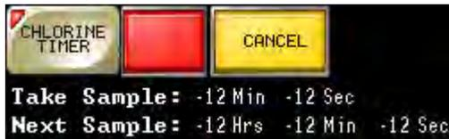
2. Once the chlorine timer has counted down (settable from 1-30 minutes), an audible alarm will sound prompting the user to collect the sample at the sample station. The screen will also display "TEST COMPLETE" and "END OF DAY" buttons.
