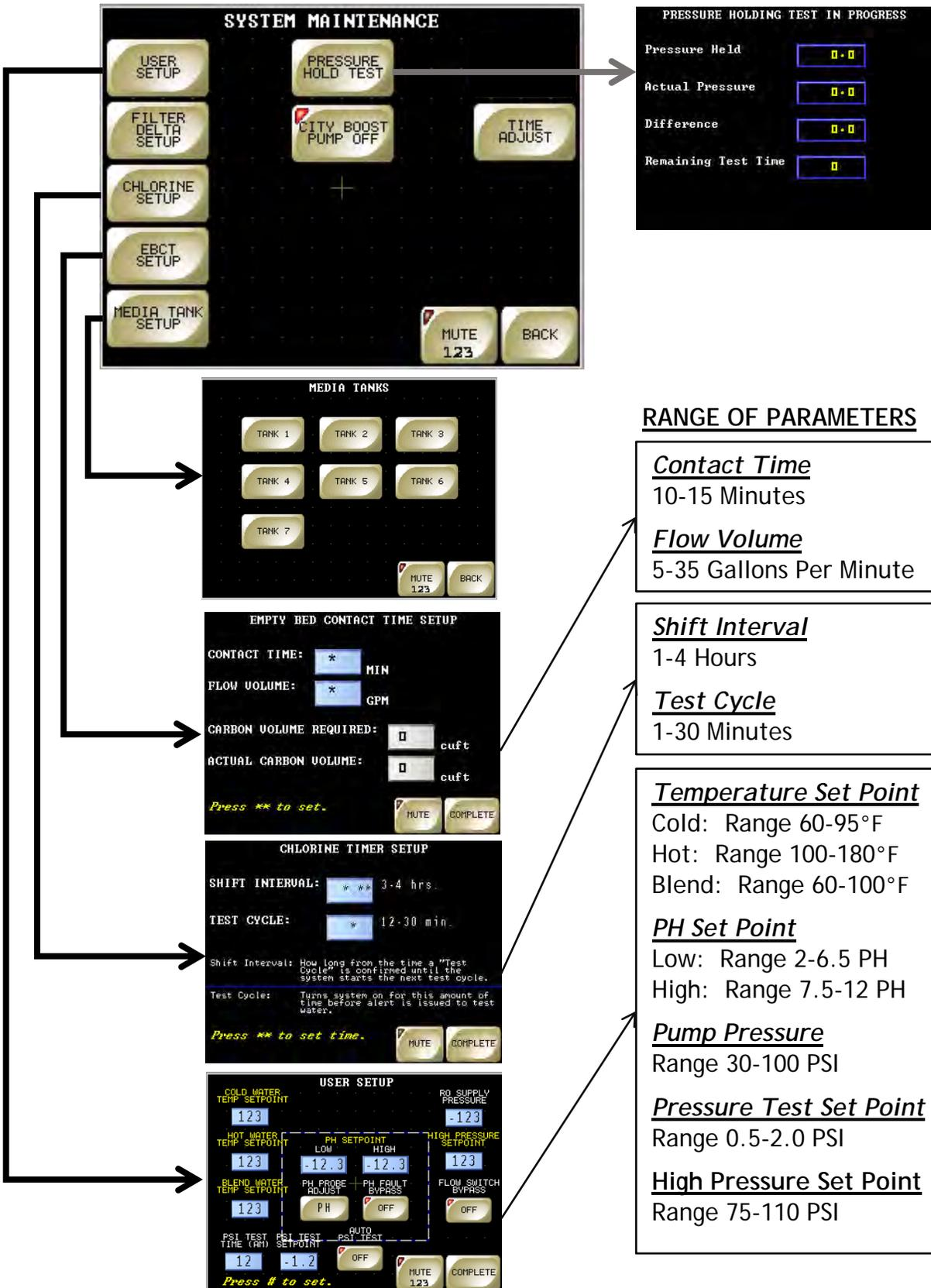
**Section 4.4****INTERFACE SETUP - USER SETUP**
