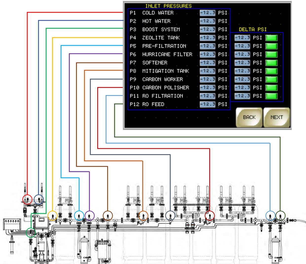
The **SYSTEM DATA** screen allows the user to monitor all pre-treatment pressures in real time. Temperatures of pre and post blending valve are monitored and displayed. Delta pressure drops across filters and media tanks are calculated and displayed in real time. Out of range Delta Pressures produce a banner alert across the OIT.
