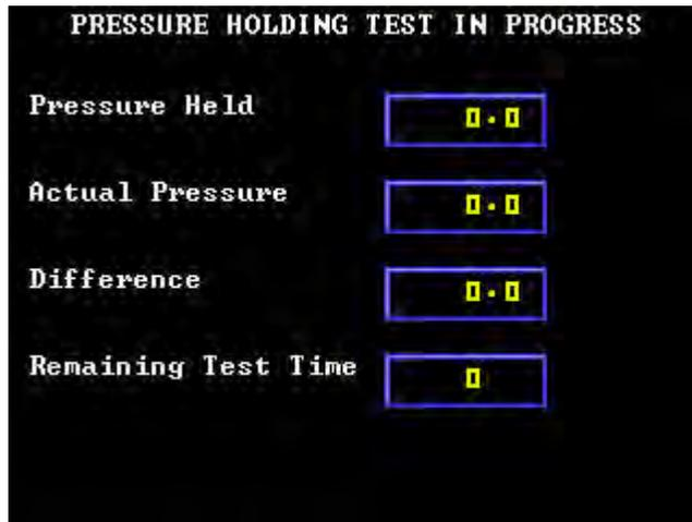
**Pressure Held:** Is the pressure the system is at when "Pressure Holding Test" was initiated.
