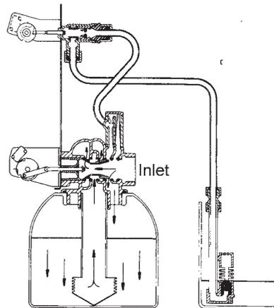
Hard water enters unit at valve inlet, flows directly from inlet down through mineral into center tube bottom distributor and up through center tube, around piston and out through the drain line.
