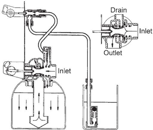
Hard water enters unit at valve inlet and flows down through the mineral in the mineral tank. Conditioned water enters center tube through the bottom distributor, then flows up through the center tube, around the piston, and out the outlet of the valve.
