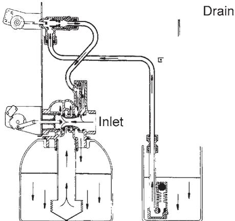
Hard water enters unit at valve inlet, flows up into injector housing and down through nozzle and throat to draw brine from the brine tank, brine flows down through mineral and enters the center tube through bottom distributor and out through the drain line.
