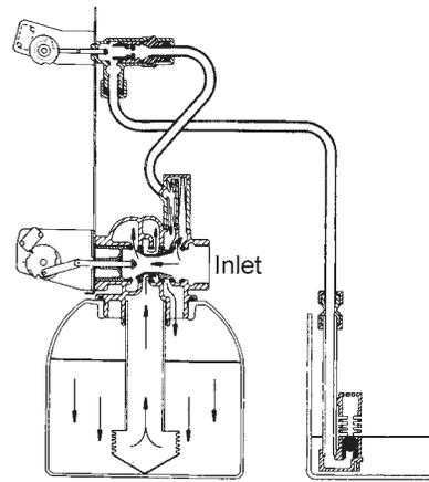
Hard water enters unit at valve inlet, flows up into injector housing and down through nozzle and throat, around the piston, down through mineral, enters center tube through bottom distributor, flows up through center tube, around piston and out through drain line.
