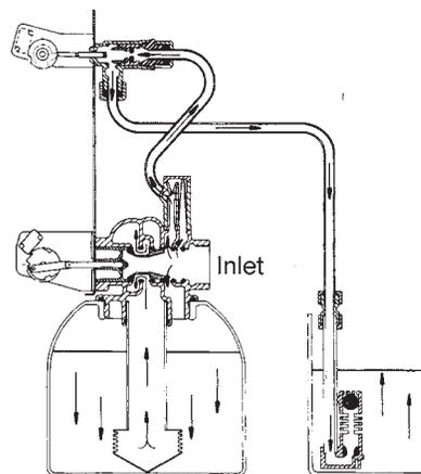
Hard water enters unit at valve inlet, flows up through the injector housing, through the brine valve to refill the brine tank.
