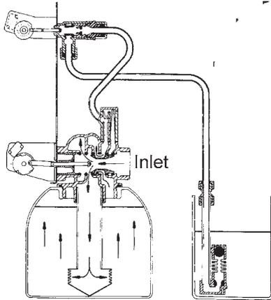
Hard water enters unit at valve inlet, flows through piston, down center tube, through bottom distributor, and up through the mineral, around the piston and out the drain line.
