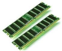
Random-access memory (RAM) -- Even the fastest processor needs a buffer to store information while it's being processed. The <u>RAM</u> is to the CPU as a countertop is to a cook: It serves as the place where the ingredients and tools you're working with wait until you need to pick up and use them. Both a fast CPU and an ample amount of RAM are necessary for a speedy PC. Each PC has a maximum amount of RAM it can handle, and slots on the motherboard indicate the type of RAM the PC requires.
