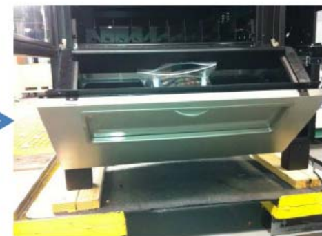
Bin tilted out to access bolts
