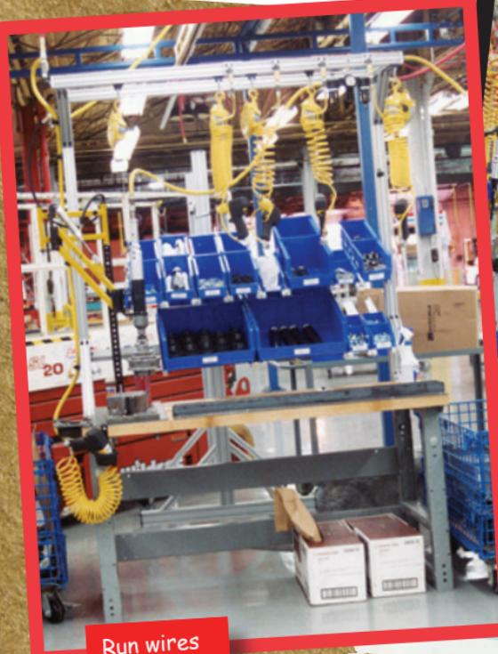
Run wires in the T-slot
