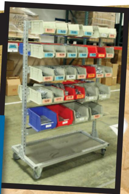
Part bins are easily mounted to T-slotted profiles.
