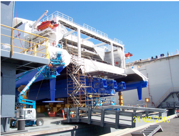
Figure 6: Transom-mounted T-foils, port and starboard, prior to trials.
