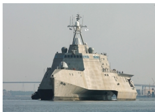
Figure 1: USS Independence, a 40-knot 126-metre trimaran designed and built by Austal
