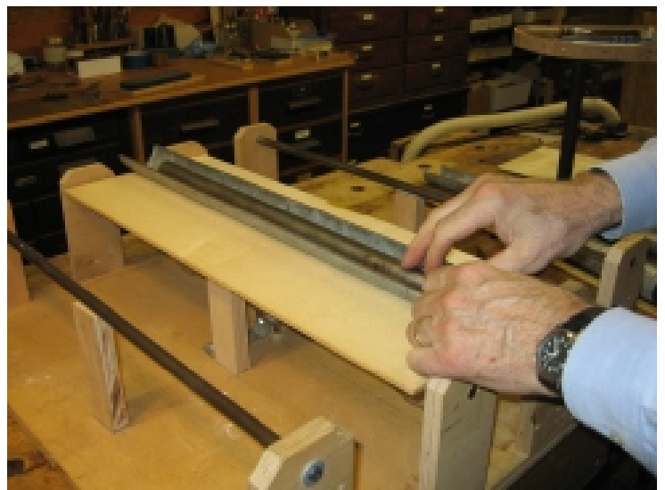
Deflection weight being put in place, and reading taken
