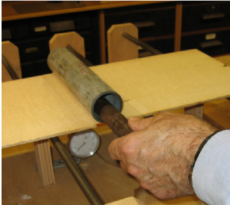
Deflection weight being put in place, and reading taken
