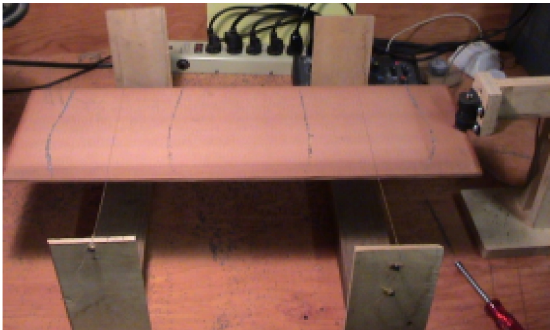
The sample is supported on threads about 20% from each end.
