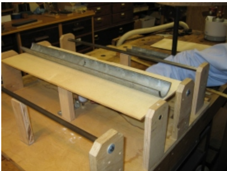
“ Biasing weight” in place, and bezel being set to zero
