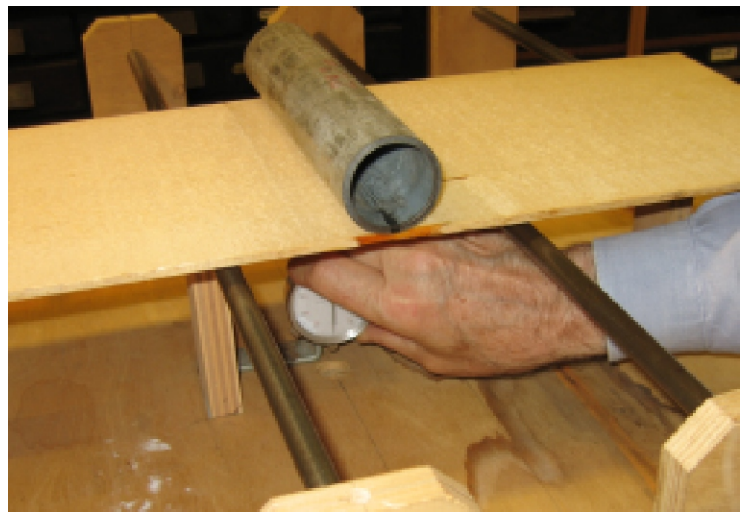
“ Biasing weight” in place, and bezel being set to zero
