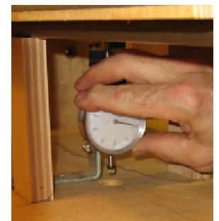
Adjusting bezel to zero
