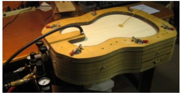
My voicing form approximates gluing the top to sides.
