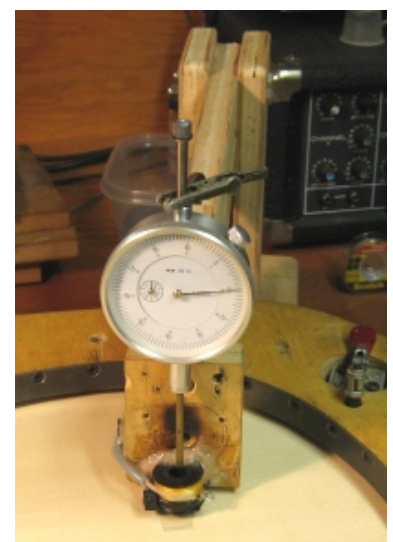
Plunger up for clearance--note alligator clip holder
