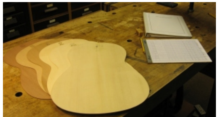
The 6 sound boards chosen for the current batch— 2 western red cedar, 1 redwood, 3 Euro-spruce
