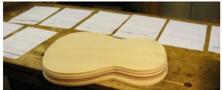
16 tops thinned to a 75 Hz monopole, with one cedar top taken down to 70 Hz for a “larger” classic.
