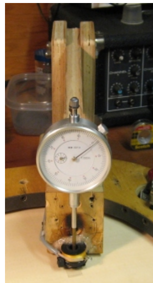
Plunger down for measurement
