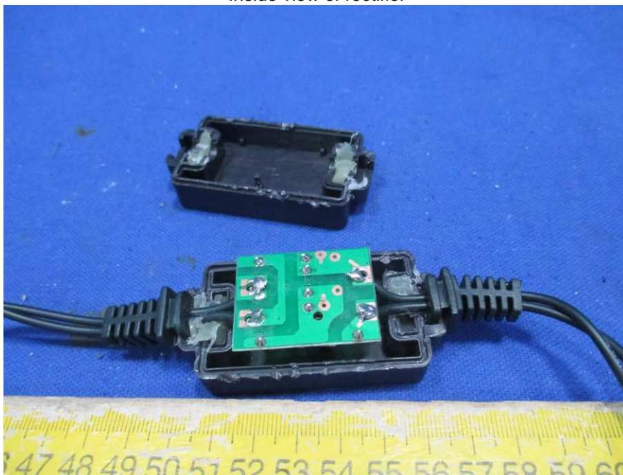
Photo 4. Inside view of rectifier
