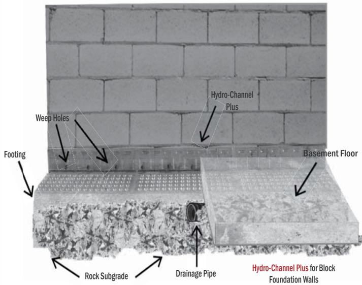
Hydro-Channel Plus for Block Foundation Walls
