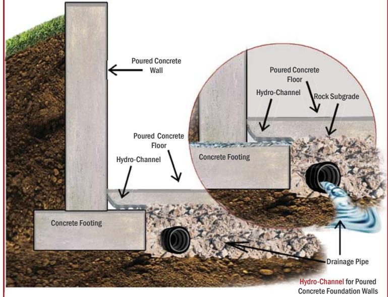
Hydro-Channel for Poured Concrete Foundation Walls
