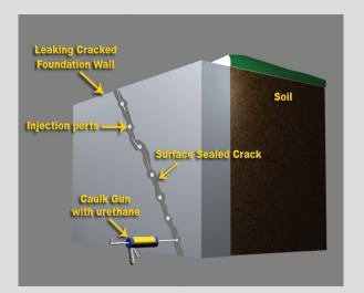
The Emecole Crack Repair System contains a very thin urethane which travels all the way through the wall. Once in the wall and beyond, it expands and plugs. The resulting foam barrier permanently stops the flow of water. The benefits of the expanding foam include:
