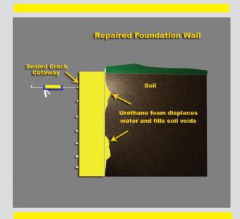
Stops leaks by searching out all voids and filling the crack completely through to the soil.
