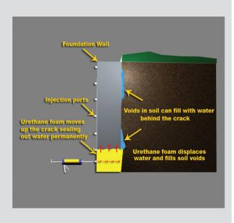
Repairing cracks is an essential step before finishing off your basement.
