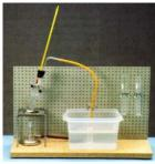
Peg Board Kit. Kit includes a pegboard back to be mounted on a base with parts included for assemblies to conduct basic experiments. Parts included are clips, standoffs, screws, washers and wing nuts.
