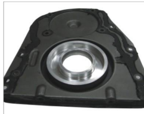
2. Take off the front part, and push the cover into the flange.
