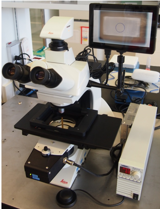
Upright microscope version of the instrument on a Leica DM2700
