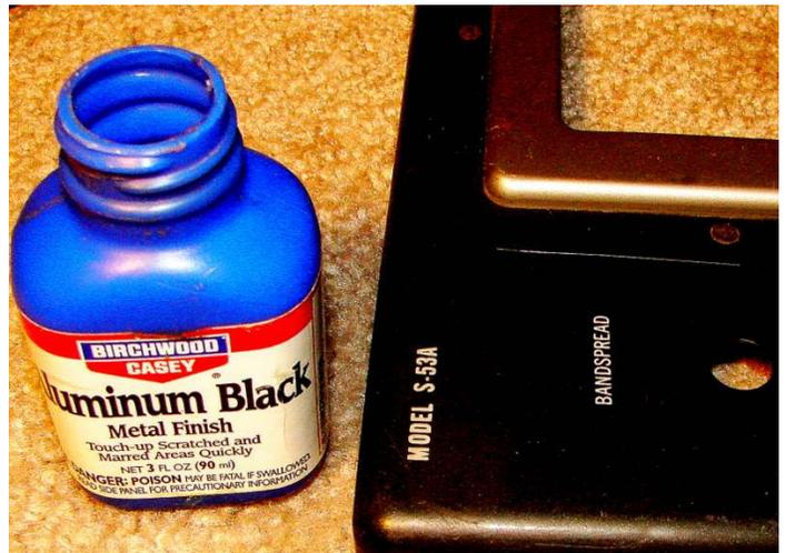
After carefully airbrushing the panel with this expensive paint, it became apparent that the entire radio would now have to be painted, since the new paint didn’t quite look right when compared to the 70 year old partially oxidized paint on the rest of the receiver! All of this, just to get rid of this two inch mar.
