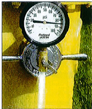
Static Fire Hydrant Gauge with Bleeder Valve takes out air and also lets you know the hydrant is draining
