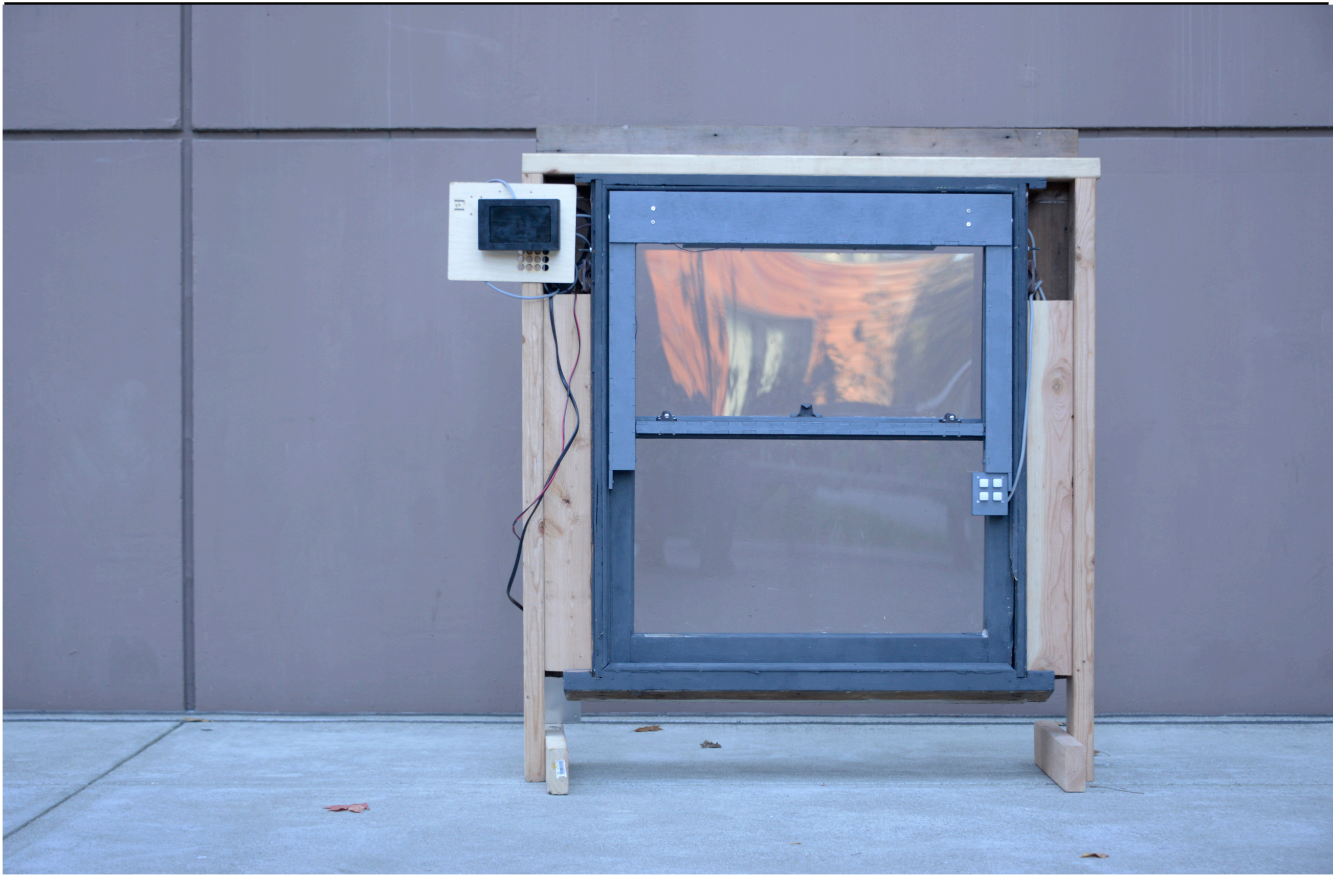
The WinDo installed on a double-hung window.
