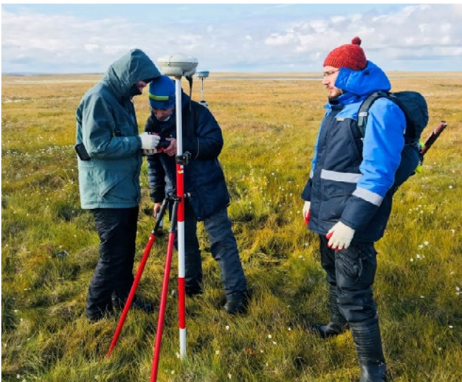
Figure 4: DGPS&LIDAR mapping of Kara sea coastal line (Isaev et al., 2019) by Norwegian student (Vadim Simonsen) supervised by MSU&ArtGeo specialists (Ruslan Amangurov&ArtGeo).
