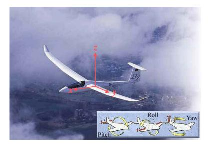
Figure 1.1. **Roll, pitch, and yaw as defined for an aircraft.** The long axis of the airplane is defined as the x-axis, the wings define the y-axis, and a line perpendicular to the plane containing the wings is defined as the z-axis. Rotation about these axes is called roll, pitch, and yaw, respectively. As the airplane maneuvers, the coordinate system remains "attached" to the airplane.
