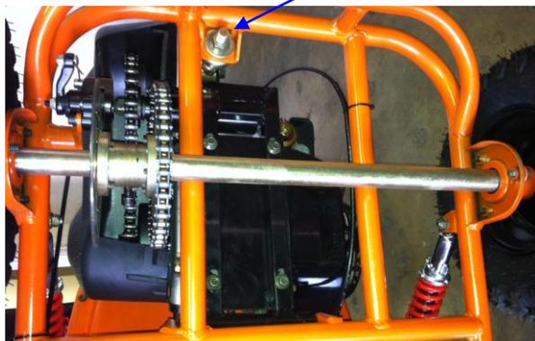
C. After the go-kart has been driven for a while, the drive chain on clutch will be loosen and should be readjusted. At first, four bolts fixing the engine on mount plate have to be loosen until the engine can be moved. Then, adjust the chain adjusting bolt at the front side of engine to tighten the chain to an appropriate tension. At last, after adjusting screw the four bolts tightly.
