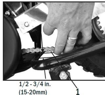
B. If after step. 1 tightening the nut of chain adjustor the chain is still too loose or too tight, another nut at the underpart of chain adjustor must be adjusted accordingly.
