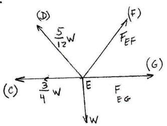
$$\frac{5}{12} W \sin \theta + F_{EF} \sin \theta - W = 0; F_{EF} = \frac{1}{\sin \theta} \left( W - \frac{5}{12} W \sin \theta \right) = \frac{5}{4} \left( 1 - \frac{5}{12} \frac{4}{5} \right) W; F_{EF} = \frac{5}{6} W \text{ tração}$$
