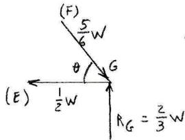
$$\left. \begin{aligned} -\frac{5}{6}W \sin \theta + R_G &= -\frac{5}{6} \frac{4}{5}W + \frac{2}{3}W = \left(-\frac{2}{3} + \frac{2}{3}\right)W = 0 \\ -\frac{1}{2}W + \frac{5}{6}W \cos \theta &= \left(-\frac{1}{2} + \frac{5}{6} \frac{3}{5}\right)W = \left(-\frac{1}{2} + \frac{1}{2}\right)W = 0 \end{aligned} \right\} \text{ verifica-se o equilíbrio em G.}$$
