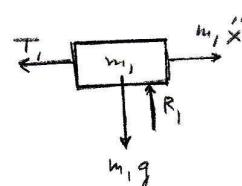
$$\begin{aligned} b) \quad & T_2 = m_3 g - m_3 \ddot{y} \\ & T_2 = T_1 + m_2 \ddot{x} \\ & T_1 = m_1 \ddot{x} \end{aligned} \quad \left. \begin{array}{l} m_3 g - m_3 \ddot{x} = m_1 \ddot{x} + m_2 \ddot{x}; \\ \ddot{x} = \frac{m_3}{m_1 + m_2 + m_3} g = \frac{2}{1+2+2} g = \frac{2}{5} g \end{array} \right\}$$
