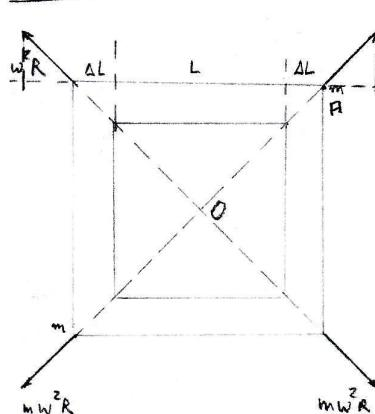
$$m\omega^2 R \cos 45^\circ = k 2\Delta L ; \quad \Delta L = \frac{m\omega^2 R}{2\sqrt{2}k}$$
