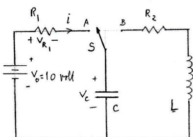
$$R_1 = 10^4 \Omega \quad C = 1 \text{ mF}$$
