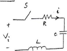
$$V_i = R i + L \frac{di}{dt} + V_C \quad e \quad i = C \frac{dV_C}{dt} \quad \text{vermos: } L C \frac{d^2V_C}{dt^2} + R C \frac{dV_C}{dt} + V_C = V_i$$
