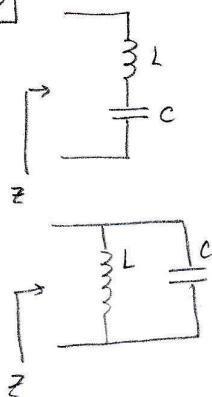
$$Z = j\omega L + \frac{1}{j\omega C} = j\left(\omega L - \frac{1}{\omega C}\right) = j \frac{\omega^2 LC + 1}{\omega C}$$
