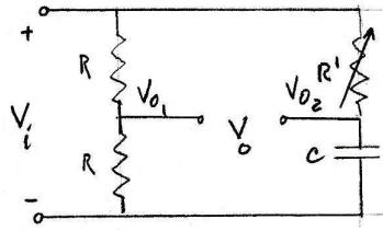
$$V_{o_1} = \frac{V_i}{2R} R$$
