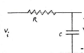
$$V_i = R i + V_c = RC \frac{dV_c}{dt} + V_c \quad \text{e } V_c = V_0 \text{ e vem:}$$
