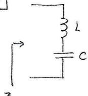
$$z = j\omega L + \frac{1}{j\omega C} = j\left(\omega L - \frac{1}{\omega C}\right) = j \frac{\omega^2 LC - 1}{\omega C}$$
