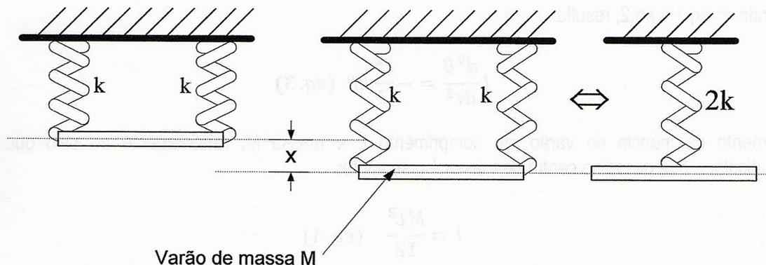
$$M \frac{d^2x}{dt^2} = -2kx \Rightarrow \frac{d^2x}{dt^2} + \frac{2k}{M}x = 0 \Rightarrow \omega^2 = \frac{2k}{M}$$
