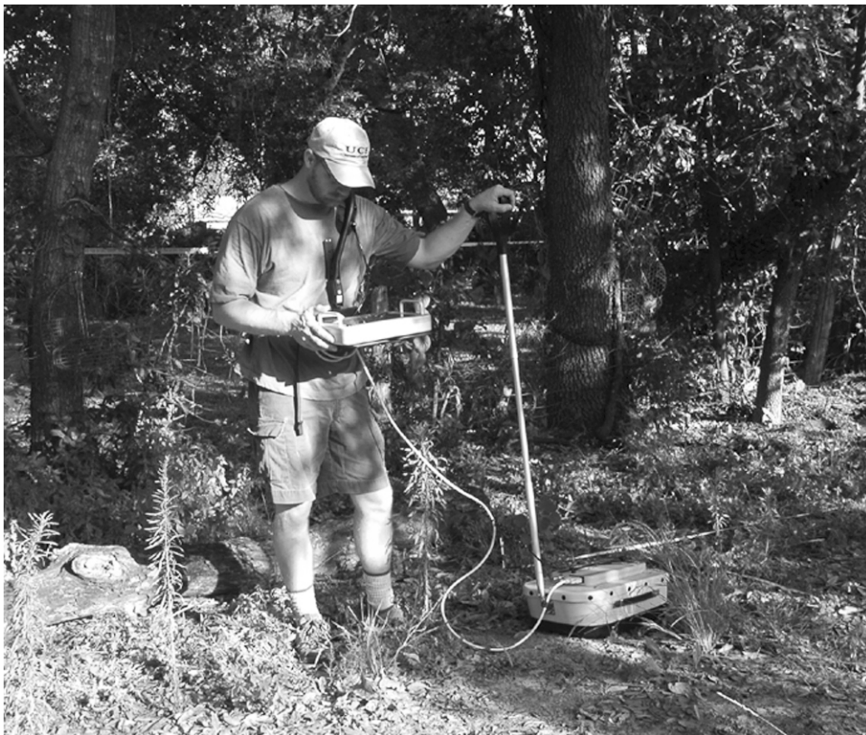
Figure 1. The author using a GPR unit at a forensic search by hand pulling the antenna across a grid.
