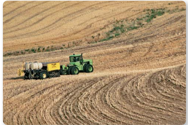
In contour plowing, crop rows are planted in curved lines along land's natural contours.
