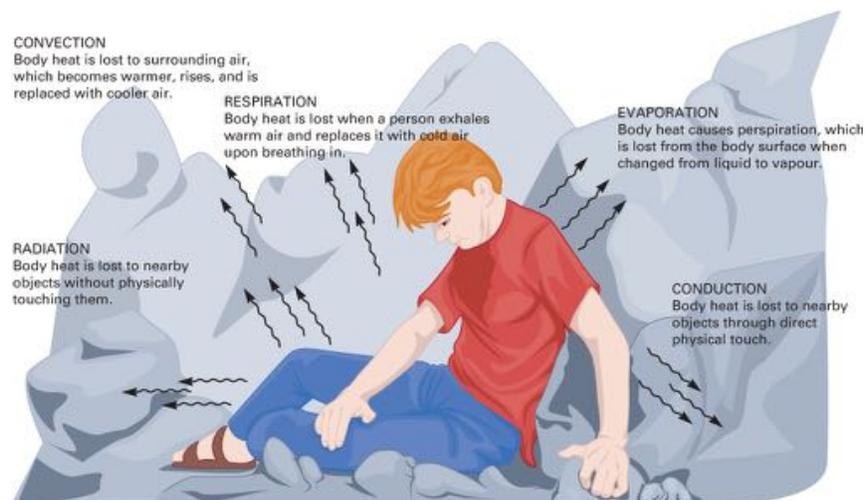
**Figure 16-1** Mechanisms of heat loss.
