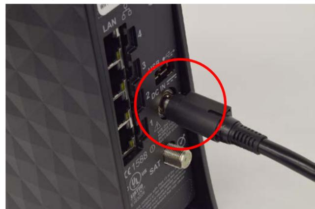
Figure 4: Incorrect power cord connection
