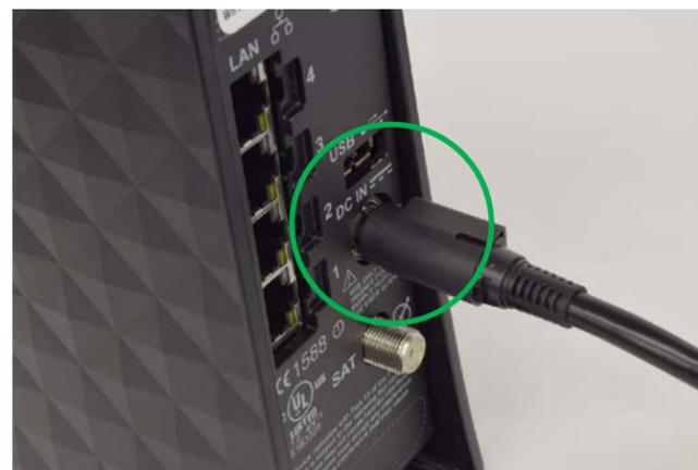
Figure 3: Correct power cord connection
