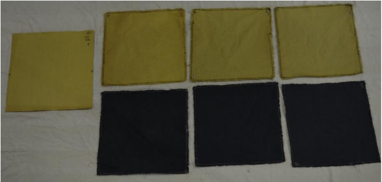
PBI Max 7.0 oz/yd 2 with Teflon FPPE (Tan and Black) LAUNDERED FABRIC SWATCHES TOP: XEROS OUTERSHELL LAUNDERING 10 CYCLES, 30 CYCLES, 50 CYCLES BOTTOM: MILNOR OUTERSHELL LAUNDERING 10 CYCLES, 30 CYCLES, 50 CYCLES LEFT: PRISTINE
