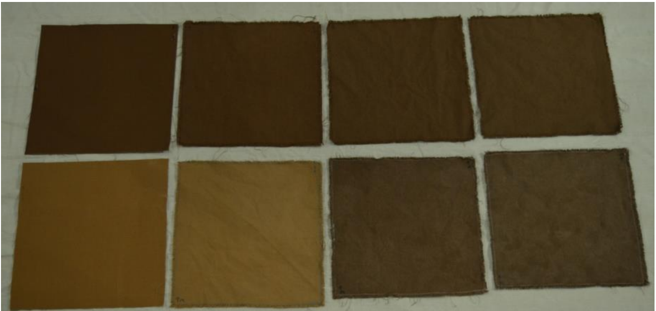
OMNI VANTAGE (LIGHT AND DARK BROWN) LAUNDERED FABRIC SWATCHES TOP: DARK BROWN PRISTINE, XEROS OUTERSHELL LAUNDERING 10 CYCLES (DARK BROWN), 30 CYCLES (DARK BROWN), 50 CYCLES (DARK BROWN) BOTTOM: LIGHT BROWN PRISTINE, MILNOR OUTERSHELL LAUNDERING 10 CYLCES (LIGHT BROWN), 30 CYCLES (DARK BROWN), 50 CYCLES (DARK BROWN)
