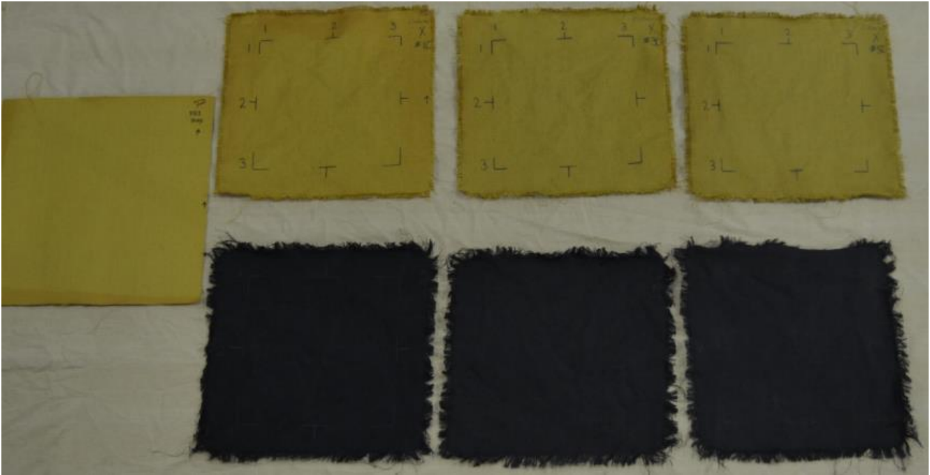
PBI Max 7.0 oz/yd 2 with Teflon FPPE (Tan and Black) CLEANING SHRINKAGE SAMPLES TOP: XEROS OUTERSHELL LAUNDERING 10 CYCLES, 30 CYCLES, 50 CYCLES BOTTOM: MILNOR OUTERSHELL LAUNDERING 10 CYCLES, 30 CYCLES, 50 CYCLES LEFT: PRISTINE
