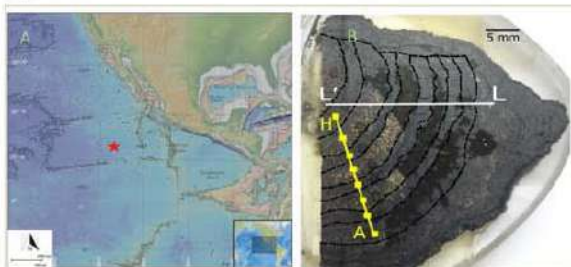
Fig.1: (A) Map showing Clarion Clipperton Zone, red star indicates the location of Fe-Mn nodule sample JC120-104B; (B) Ferromanganese nodule sample embedded in the resin. L-L' line shows the \mu -XRF (micro-X Ray Fluorescence) analysis profile, while A-A' line shows the location of sub-samples (about 2mm cubes) collected for rock magnetic studies.
