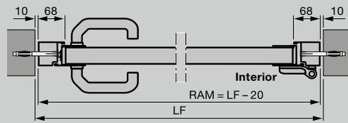
Side door with aluminium block frame, profile type 2
