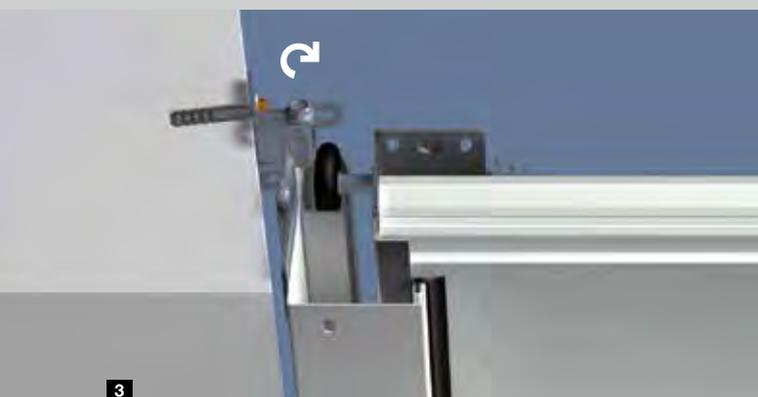
4 Fitting with non-load bearing facades (facing brick or thermal insulation) with at least 90 and max. 125 mm sideroom
